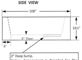
Siphon Arrangement Is Provided For The Removal Of Rain Water & Spilled Petroleum Products.
